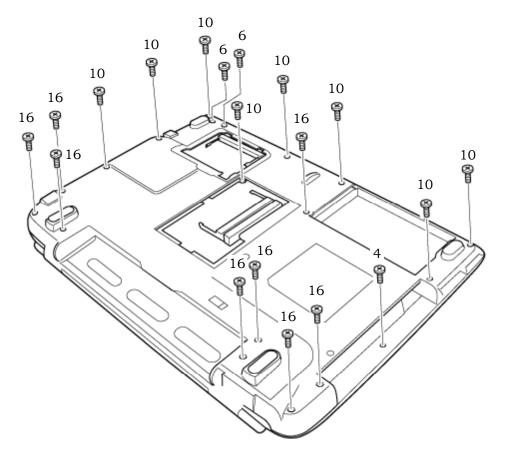
Figure 4-15 Removing the display assembly (1)
